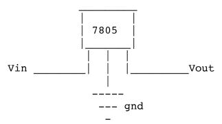
Vin = Voltage in, 6-12 volt wall adaptor, + goes to Vin, goes to gnd
